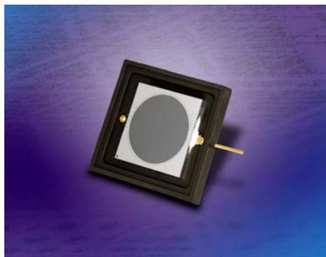
Opto Diode's high-speed photodiode is shipped with a cover plate to protect the photodiode chip and the wire bonds. Storage and operating temperatures range from -10 °C to +40 °C (ambient) and from -20 °C to +80 °C in nitrogen or vacuum environments. The lead soldering temperature is 260 °C.
